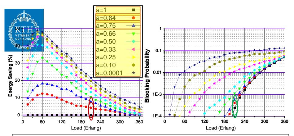
"Cost" of the link: use  $C_{link} = a_{link}^* E_{link}$ , where  $0 \le a_{link} \le 1$ ,  $E_{link} = energy$  consumption of a link; not in use  $C_{link} = E_{link}$
