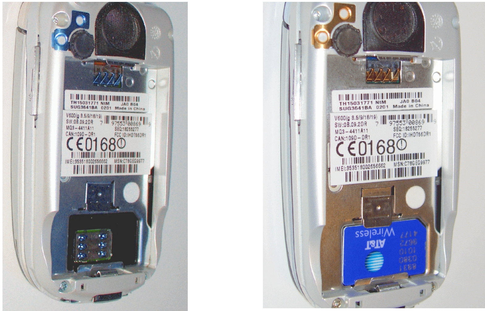
Figure 26: Phone without and with SIM card, note the IMEI number and other numbers printed inside the back of the phone.
