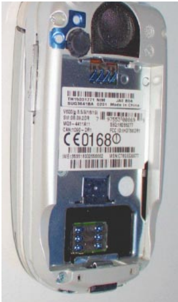
Figure 26: Phone without and with SIM card, note the IMEI number and other numbers printed inside the back of the phone.
