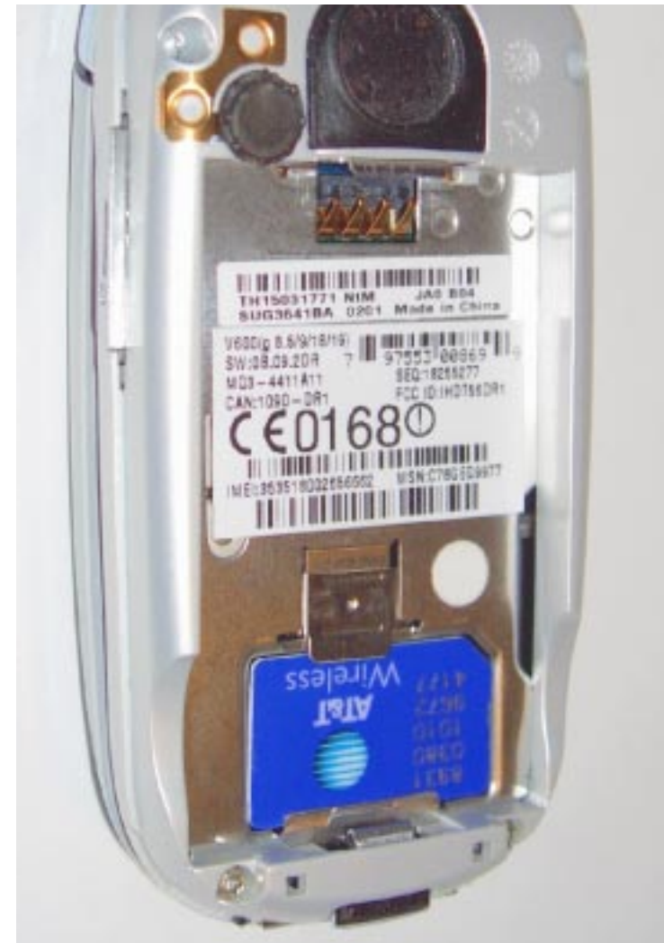
Figure 26: Phone without and with SIM card, note the IMEI number and other numbers printed inside the back of the phone.
