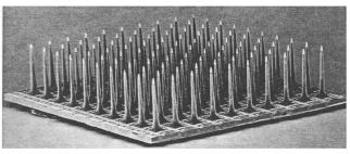
10 x 10 silicon electrode array (each electrode: 1.5mm long, 0.08mm wide at base, 0.001mm tip), Built at the Univ. of Utah, by Richard A. Normann, et al.; from Scientific American, March 1994, pg. 108.
