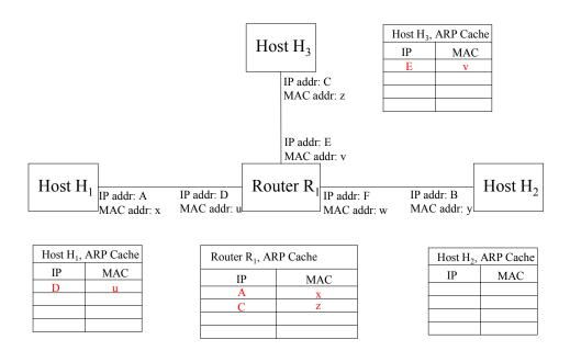
The figure above illustrates three hosts  $H_1$ ,  $H_2$  and  $H_3$  running IPv4 over a routed network, connected by router  $R_1$ . The IP and MAC addresses of the hosts and the router's interfaces are given in the figure. The ARP cache of each host and the router are shown. Assume the ARP caches are initially empty, and that no packets have been sent yet. Now, host  $H_1$  wants to send an IPv4 unicast datagram to host  $H_3$ .
