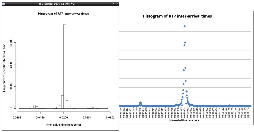
hist(To\_Chip\_RTP\_delay, ylab="Frequency of specific interarrival time", xlab="Inter-arrival time in seconds", main="Histogram of RTP inter-arrival times", breaks=46)
