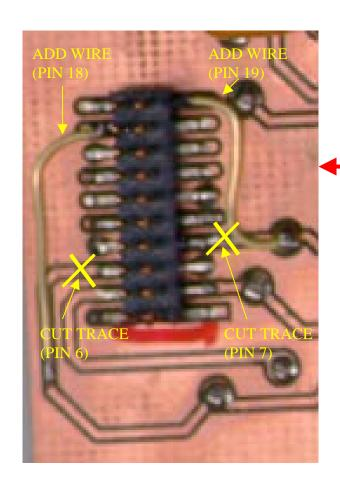
To modify the SmartBadge RS-232 buffer module to support ANGEL, you need to cut two traces and add two wires as shown above.
