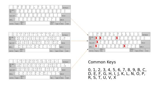
Figure 3.3. MEBx common keys (adapted from [68])
