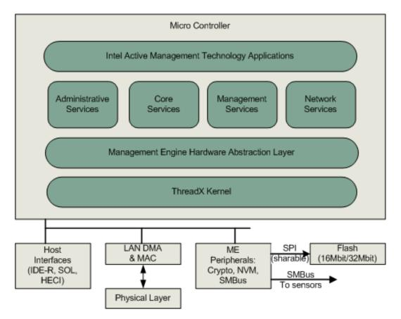
Figure 2.2. Management engine diagram in greater detail (adapted from [37])
