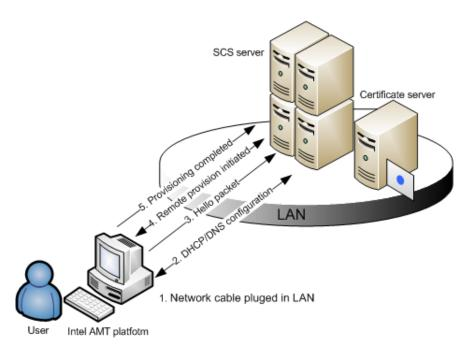
Figure 3.4. ZTC provisioning process
