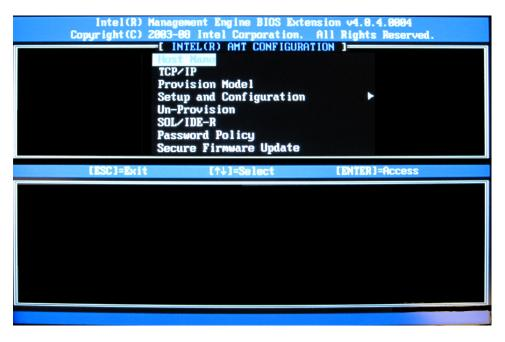
Figure 2.9. AMT MEBx configuration menu screen
