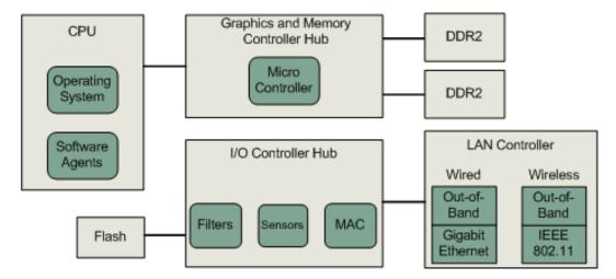
Figure 2.1. Intel AMT silicon architecture (adapted from [37])
