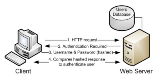
Figure 3.2. Digest access authentication schema
