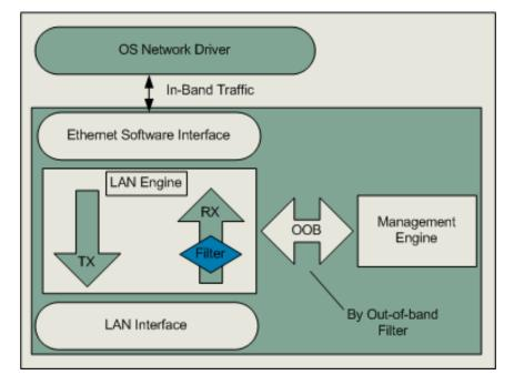
Figure 2.6. Routing local requests to Intel AMT (adapted from [52]
