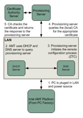
Figure 3.5. AMT provisioning flow
