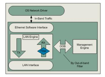
Figure 2.3. Management engine network OOB architecture (adapted from [37])
