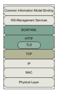
Figure 2.5. Standard management protocol stack
