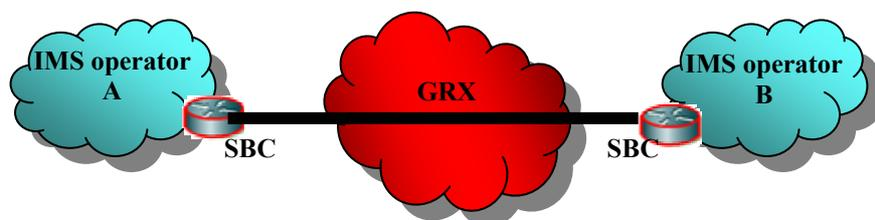
Figure 30. Interworking connection between two mobile IMS domains with SBC.
