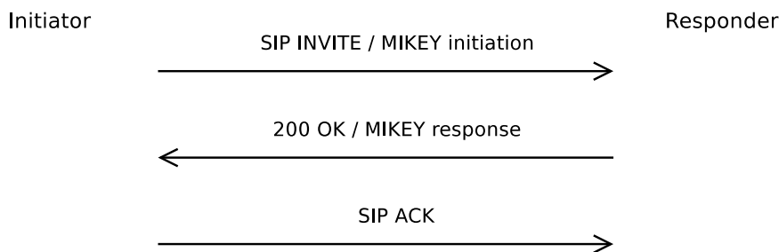
Figure 11.1: MIKEY in a SIP INVITE transaction
