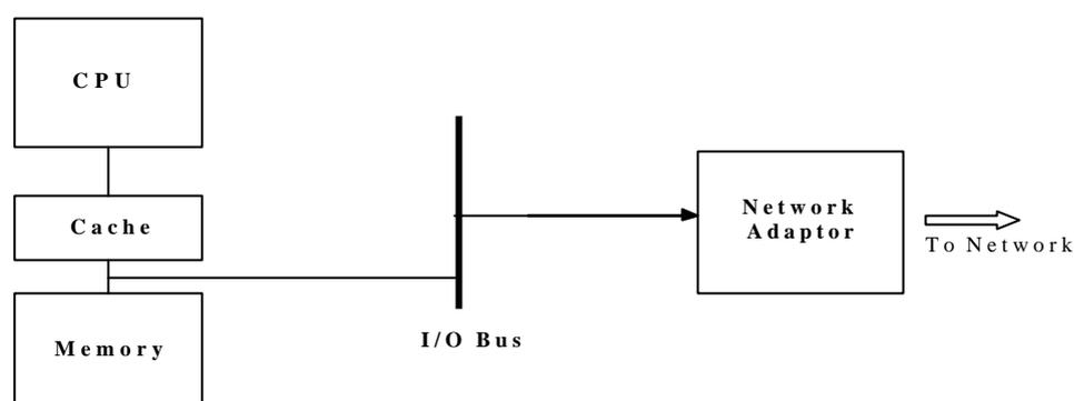
**Figure 6-1** The architecture of a host containing a network adaptor.
