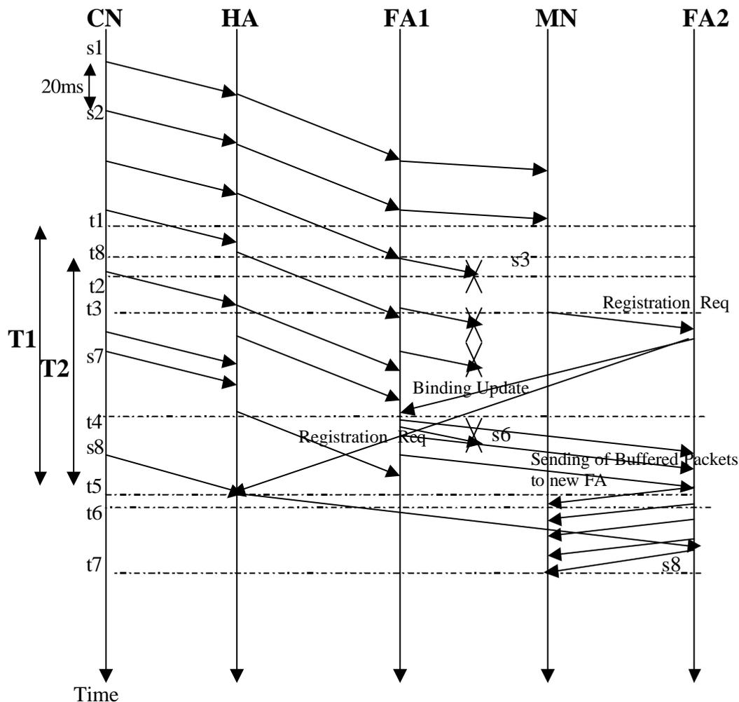
Figure 7-3 Time Sequence graph of the MIP Handoff Scenario in the case of no cell overlaps.
