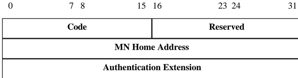
**Figure 5-7 Binding Acknowledgement Message Format.**
