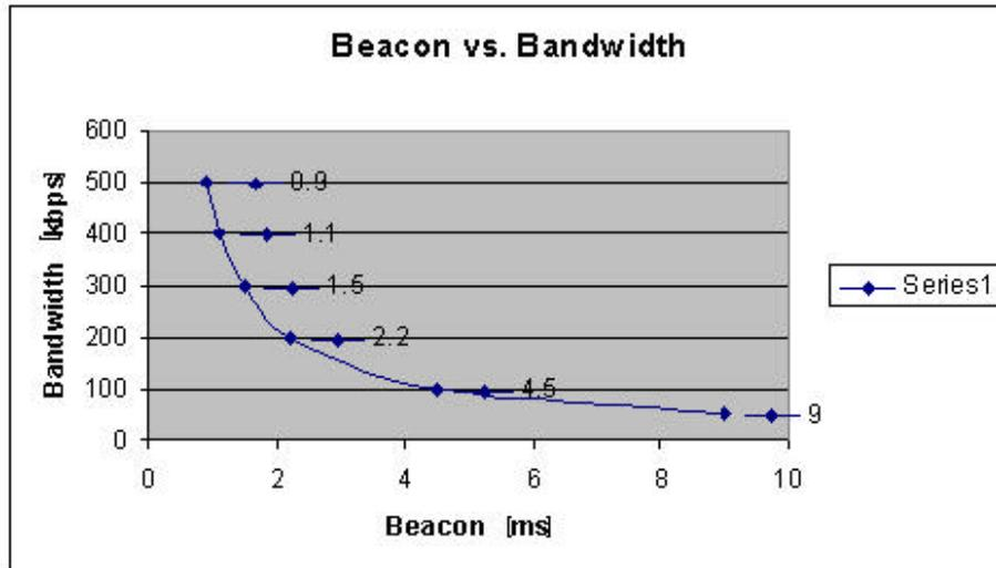
Figure 7-6 The bandwidth as a function of the beacon period
