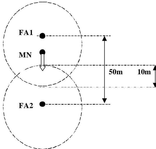
Figure 7-2 Overlap between adjacent cells.
