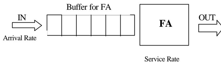
**Figure 6-7** The connection between the arrival- and service rate and the buffering scheme at the FA .
