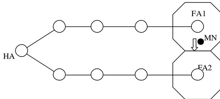
**Figure 7-7 Our wired network consists of 4 hops between the HA and FA1 and FA2.**
