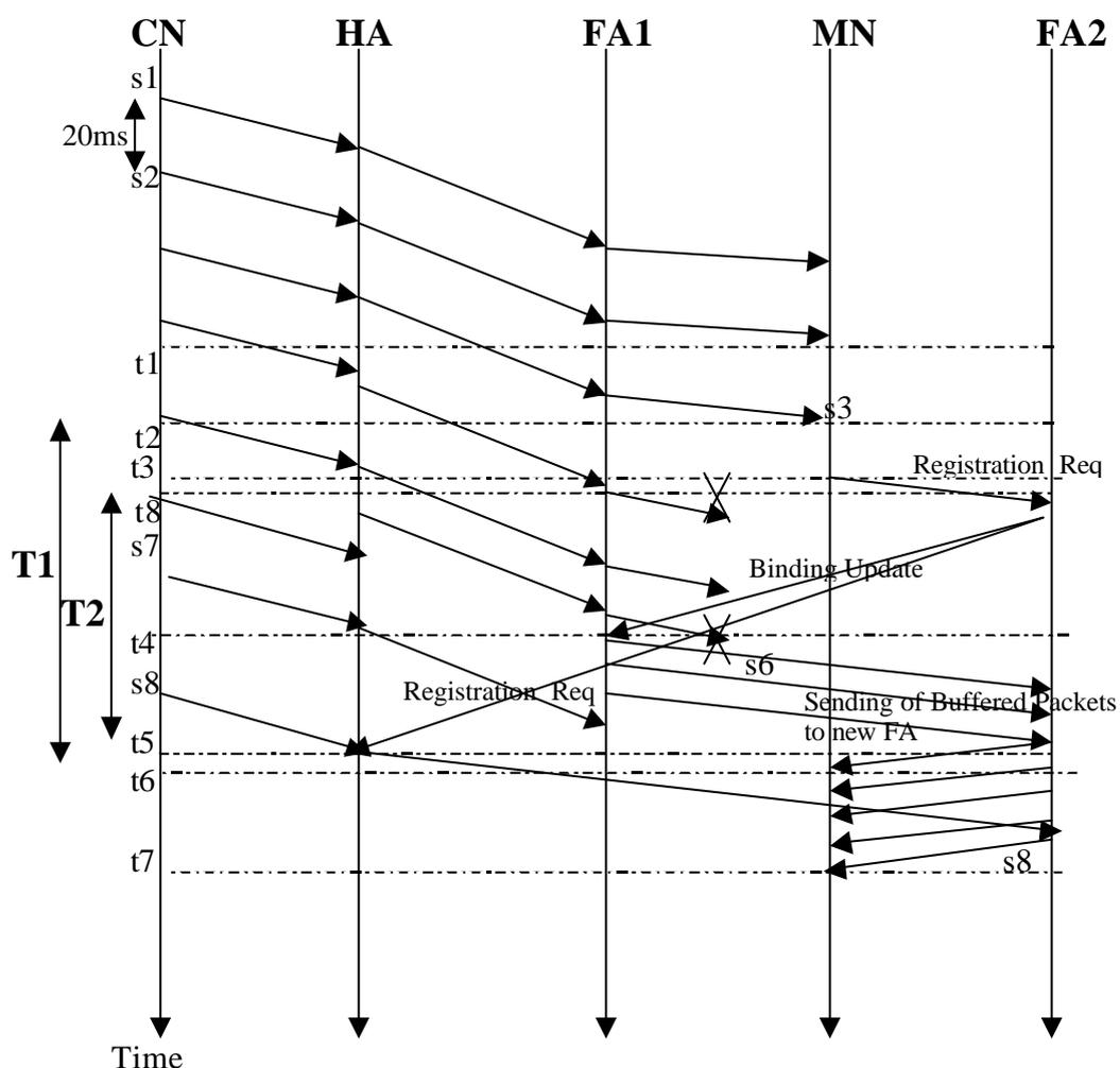
Figure 7-4 Time Sequence graph of the MIP Handoff Scenario when cells overlap.
