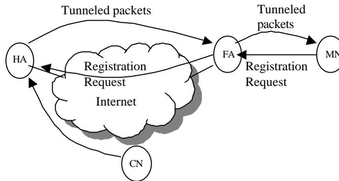
Figure 2-1 MN moving to a foreign network in Mobile IP.
