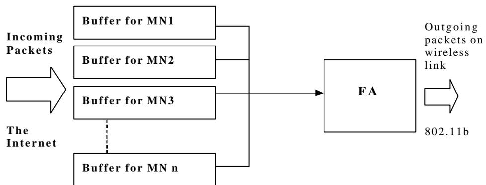
**Figure 6-5** The Scheme of having one Buffer for every MN.
