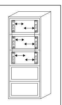
**Figure 6.1** An AXE cabinet. Each SCB of an SCB pair is responsible for about half of the boards between them.
