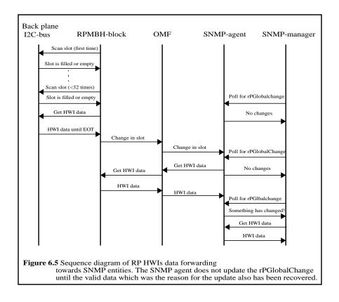
Figure 6.5 shows what happens when a new board has been put in a magazine and the RPMBH block on the SCB is made aware of it.
