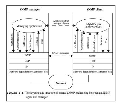
IP-protocols should be, and easy to use. SNMP doesn't necessarily need IP nor UDP as the underlying layers to function, but this is usually the case (see Fig. 5.5).
