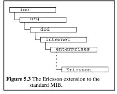
The MIB-tree was developed to support simplicity and the possibility of extending the tree
