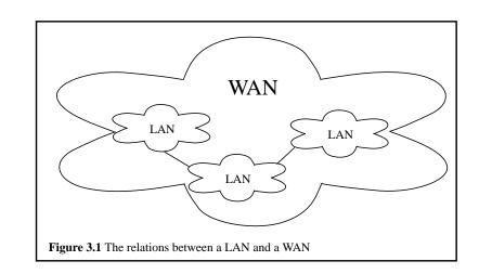
ings. A WAN is usually built from of a number of LANs that are interconnected
