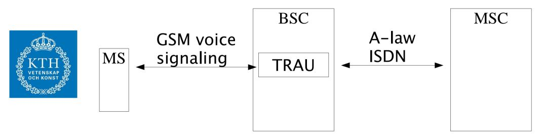
The TRAU needs not only the 13kb/s voice stream but also BFI information etc. 3 kb/s signaling and error detection is added resulting in a 16 kb/s stream.
