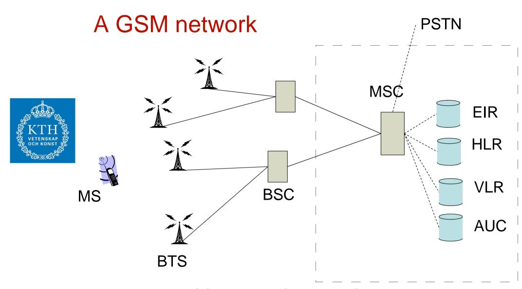
MSS – Mobile Switching Subsystem
