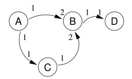
Figure 5: A synchronous data flow process network
