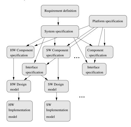
Figure 2: A SoC Design Process involves many models.
