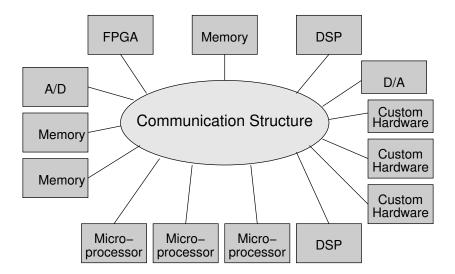
Figure 1: A possible system-on-a-chip architecture
