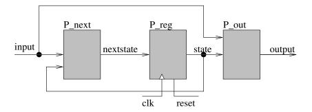
Figure 8: A VHDL synthesis tool derives a state machine when the VHDL description contains three properly modeled processes. P\_next is a combinatorial process defining the next state transition function. P\_reg is a register storing the state. P\_out models the output encoding function.
