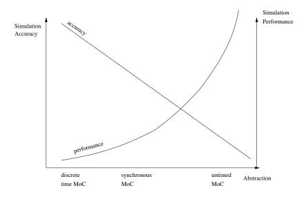
Figure 11: The trade-off between accuracy and simulation performance.
