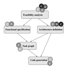
Figure 6: Suitability of MoCs in different design phases. "C"stands for continuous time MoC; "D" for discrete time MoC; "S" for synchronous MoC; and "U" for untimed MoC. More than one label on a design phase means, that all of the MoCs are required since no single MoC is sufficient by itself.
