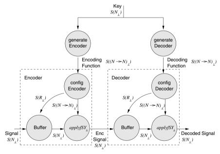
Fig. 12. The refined model of the Encoder/Decoder example takes adaptation time into account. Buffers are introduced and signal types are extended to contain the absent value, since the adaptive process cannot process any data during adaptation. The types of all signals are shown in the figure.
