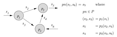
Fig. 3. A process network can be expressed by a set of equations.
