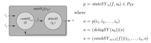
Fig. 6. The process constructor  $stateSY_n$  creates a synchronous process that models a state machine without output decoder.
