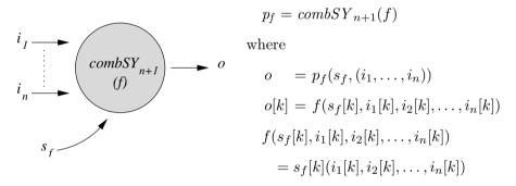
Fig. 10. The process  $applyfSY_n$  can be created be means of the process constructor  $combSY_{n+1}$ .
