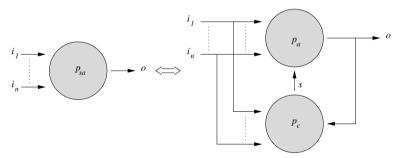
Fig. 8. A self-adaptive process is modelled as a process network of an adaptive process and an additional process. The signal s can either carry modes, functions or entire processes as illustrated in Figure 7.
