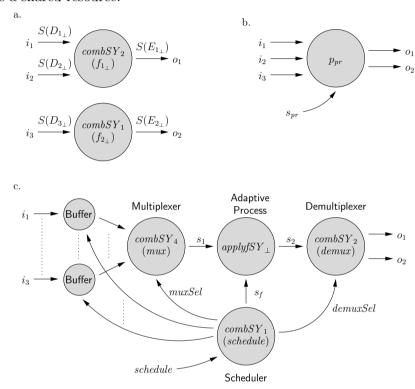
Fig. 13. Figure 13 illustrates the use of an interfaces adaptive process for resource sharing. The processes  $combSY_2(f_{1_{\perp}})$  and  $combSY_1(f_{2_{\perp}})$  shall use the adaptive process as shared resource (Figure 13a). Figure 13b shows an interface adaptive process that is configured by a signal carrying processes as signal values. Figure 13c shows a refined model using a function adaptive process, buffer processes, scheduler, multiplexer and demultiplexer processes.
