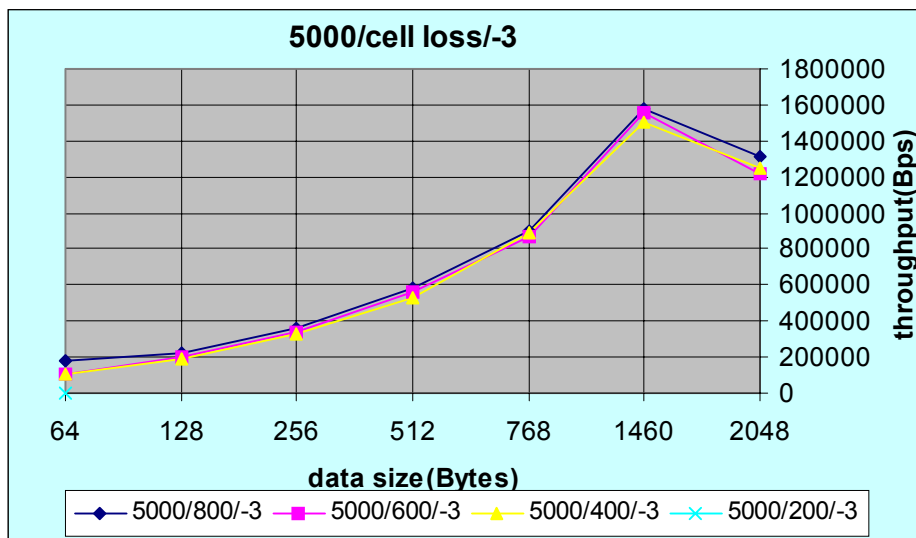
FIGURE 19. THROUGHPUT WITH CELL LOSSES.
