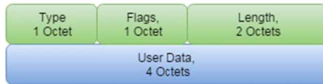
Figure 2-9: SCTP Chunk layout
