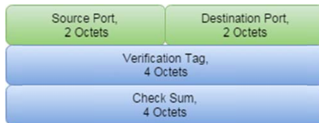
Figure 2-10: SCTP Common Header
