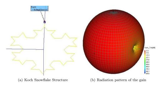
Figure 3.15: Koch Antenna second iteration,  $30 \text{ cm} \ge 30 \text{ cm}$
