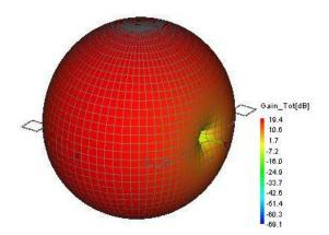
Figure 3.20: Minkowski Antenna second iteration, 40 cm x 40 cm: Radiation pattern of the gain
