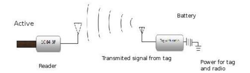
Figure 2.3: Active Tag Power/Transmit Configuration (Adapted from figure 2.16 in [1])
