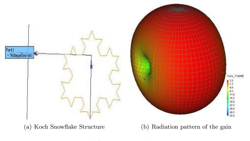
Figure 3.14: Koch Antenna second iteration, 2 m x 2 m
