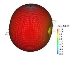
Figure 3.22: Minkowski Antenna second iteration,  $60 \text{ cm} \ge 60 \text{ cm}$ : Radiation pattern of the gain
