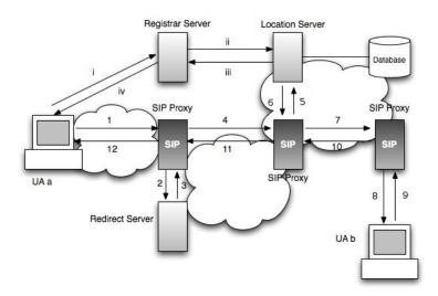
Figure 2.6: SIP Architecture and Operations (Adapted from figure 2.7 in [3])
