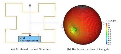
Figure 3.16: Minkowski Antenna first iteration, 2 m x 2 m
