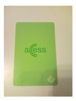
Figure 1.1: An example of an RFID Tag. This is an Access card issued by Stockholm County's public transport authority (SL)
