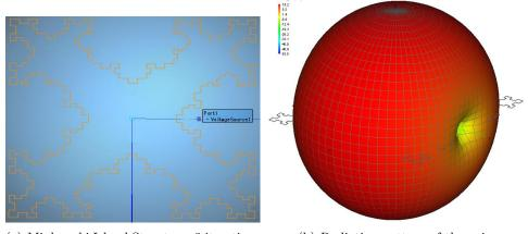
(a) Minkowski Island Structure, 3 iterations (b) Radiation pattern of the gain
