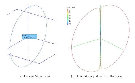
Figure 3.2: Dipole Antenna
