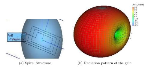
Figure 3.5: Spiral Antenna
