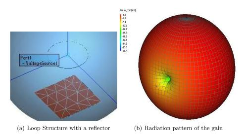
Figure 3.9: Loop with a reflector at  $\lambda/32$
