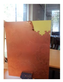
Figure 4.5: Process to remove the remaining copper from the copper clad board
