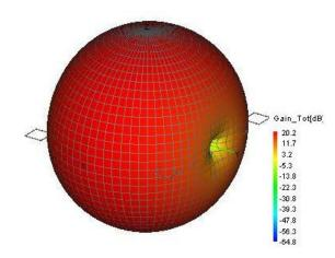
Figure 3.21: Minkowski Antenna second iteration, 50 cm x 50 cm: Radiation pattern of the gain
