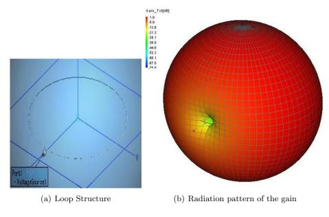
Figure 3.4: Loop Antenna
