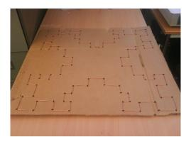
Figure 4.1: Prototype of Minkowsky Island second iteration 60cm x 60cm antenna
