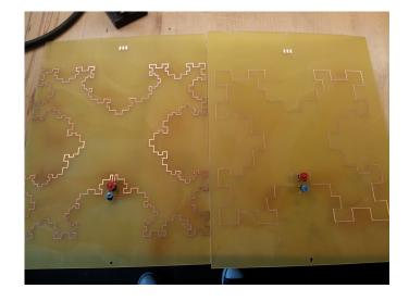
Figure 4.6: PCB Minkowski antennas for 3 and 2 iterations
