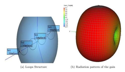
Figure 3.6: Array Loop
