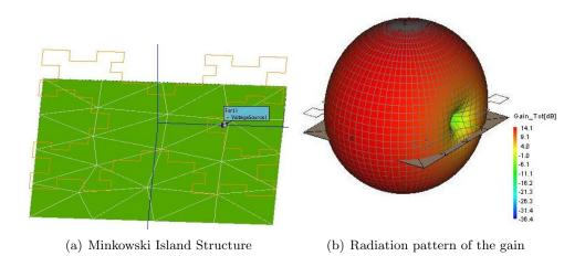
Figure 3.23: Minkowski Antenna second iteration, 60 cm x 60 cm with a reflector at  $\lambda/4$
