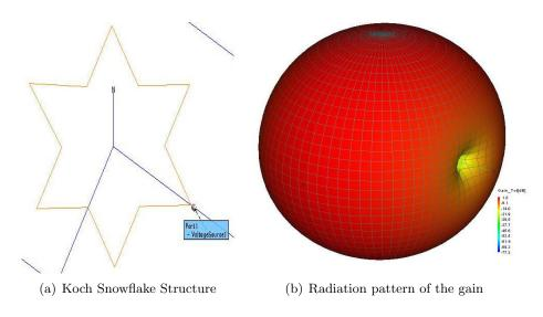
Figure 3.12: Koch Antenna first iteration, 2 m x 2 m
