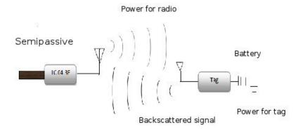
Figure 2.4: Semi-Passive Tag Power/Transmit Configuration (Adapted from figure 2.16 in [1])
