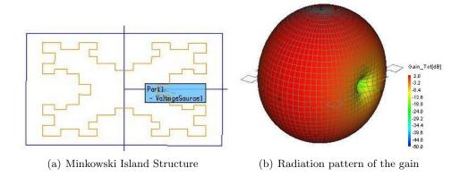
Figure 3.18: Minkowski Antenna second iteration, 2 m x 2 m
