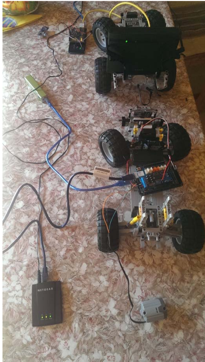
Figure 3-9: Setup of simple signals test. Front model with router and servo. Rear model with access point, servo motor, USDR sensor, and motor. Figure 3-7 and Figure 3-8 shows the blueprints for each of these.
