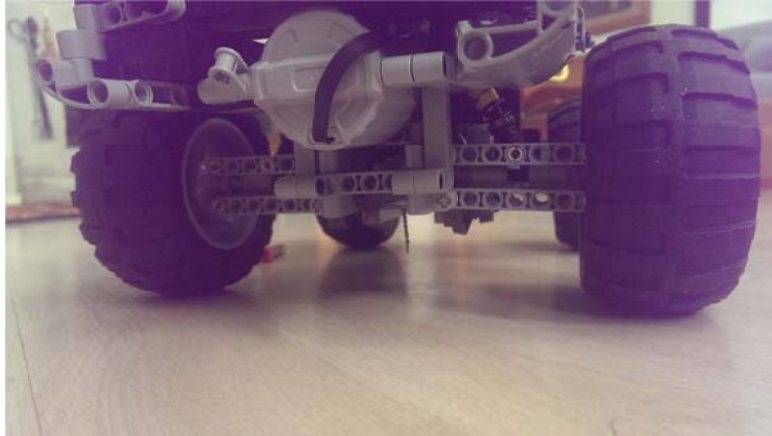
Figure 4-12: The rear axle is horizontal due to the retracted suspensions, because of the weight.
