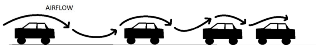
Figure 1-1: Airflow with large and small inter-vehicle separation
