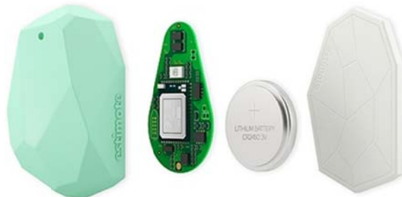
Figure 4-1: Estimote Beacon. The community manager of Estimote granted permission (by E-Mail) for use of this image in this thesis[19].
