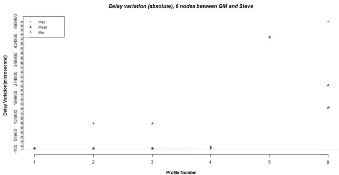
Figure 5-29: Absolute value of delay variation – six nodes between GM and slave
