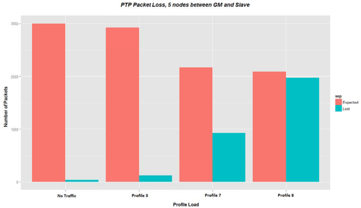
Figure 5-6: Packet loss in different profiles, five nodes between GM and slave
