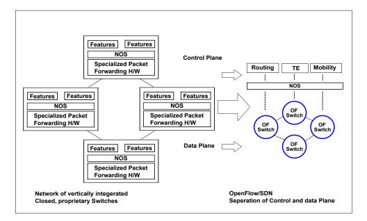
Figure 1.1: Traditional switches verses OpenFlow/SDN switches
