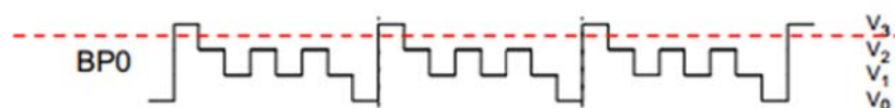
Figure 11-2: Backplane sampling trigger. It triggers when the line is at its peak.
