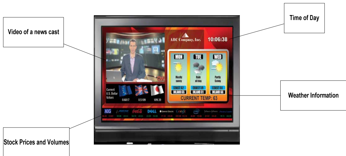
Figure 2-4: Display showing multiple zones [8] (Appears here with the permission of Taxes Digital*)
