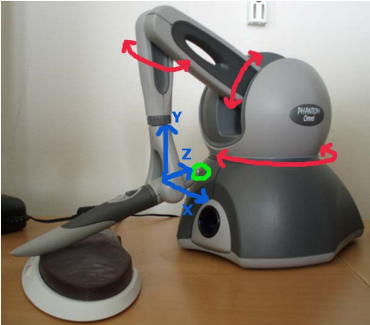
Figure 2: PHANTOM Omni with illustrated force components and possible movement of arms
