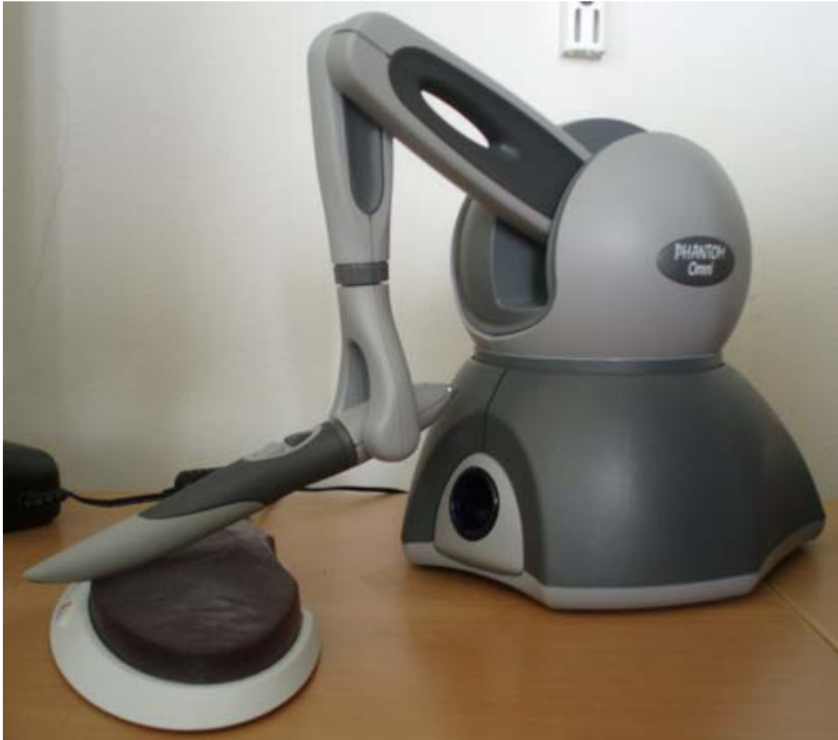
Figure 1: Photo of the PHANTOM Omni Haptic Device
