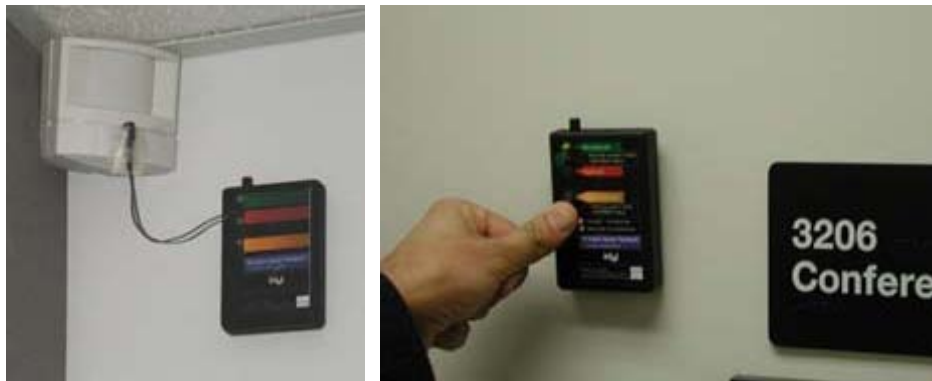
Figure 2.10 Conference Room Motion Sensor Node and Reservation Status Indicator (These figures appear here with permission from W. Steven Conner, the author of [38])
