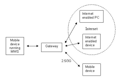
Figure 3.1. The MWS's communication paths (adapted from figure in [41]).
