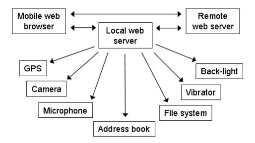
Figure 5.1. Final system structure. Web content can be loaded via the local server.
