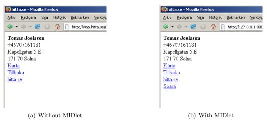
Figure 5.2. The mobile web site Hitta.se displaying details of a person. The MIDlet adds an additional link to the page. Clicking "Spara" will save the contact details to the phone's address book.
