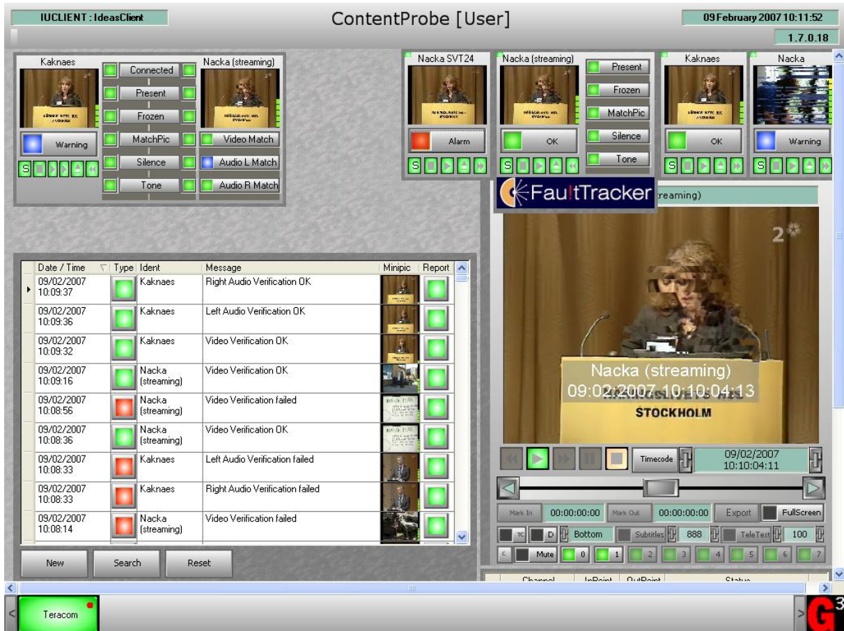
Figure 20: Client PC software displaying content with visible bit errors (Nacka (streaming)), but classified by the equipment as matched video content; shown in the top left corner of the figure. The green colored boxes in the figure indicate a correct detection, while the blue colored icons indicate events that need attention from the user. The four boxes in the top right corner of the screen shot show the different inputs to the system.
