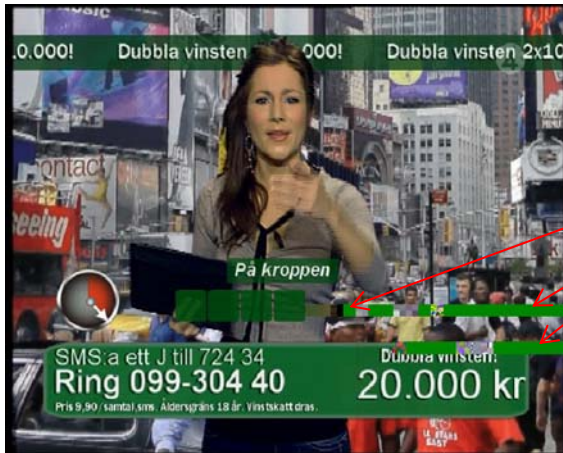
Figure 27: Screen shot from a video with bit error, represented as green blocks. (TV4).
