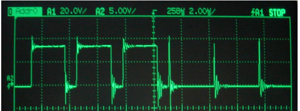
Figure 5: NDRV ON at 75% Duty Cycle (left); spikes when NDRV should be OFF (right)
