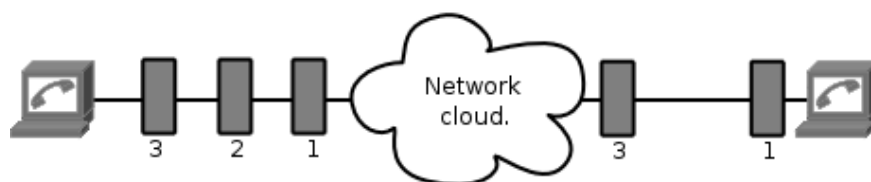
Figure 1.5: Network congestion or link failure can result in packet loss, a situation in which packets are lost on the transmission path.
