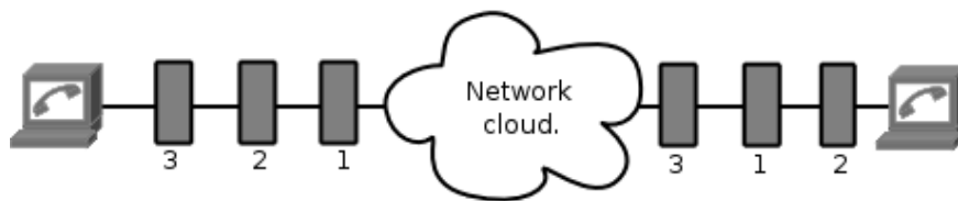
Figure 1.6: Sequence numbers help the receiver identify the correct order of packets. Media protocols such as Real-time Transport Protocol (RTP), include sequence numbers in their headers.
