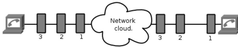
Figure 1.4: Variation of packet interarrival time, also known as jitter. A network cloud, as used in this study represents a network path with an arbitrary number of network devices such as routers and switches between its entry and exit points.
