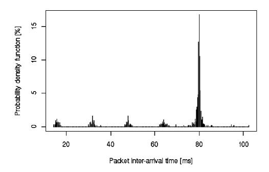
Figure 21. Quake 4 downlink packet inter-arrival time distribution
