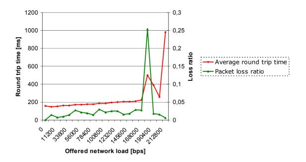
Figure 30. Large packet traffic's influence on in an EDGE network
