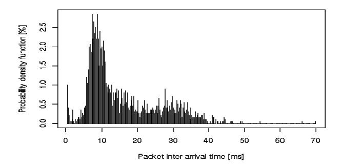
Figure 17. Quake 4 uplink packet inter-arrival time distribution
