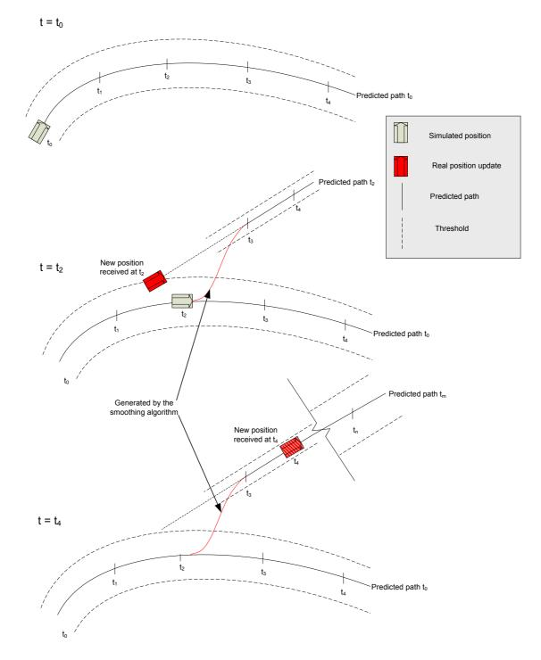
Figure 3. Dead reckoning with smoothing algorithm
