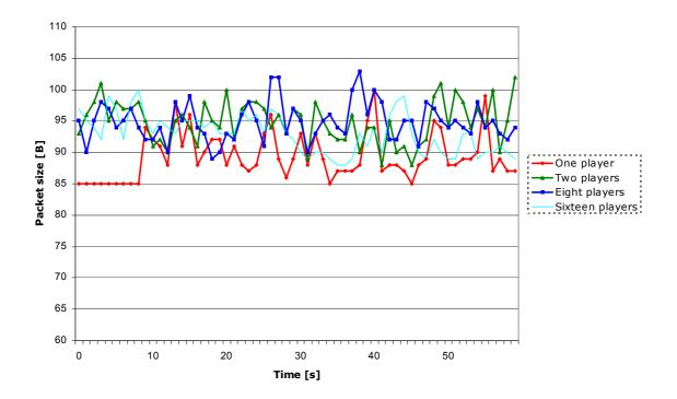
Figure 24. Quake 4 uplink packet size with varying number of players
