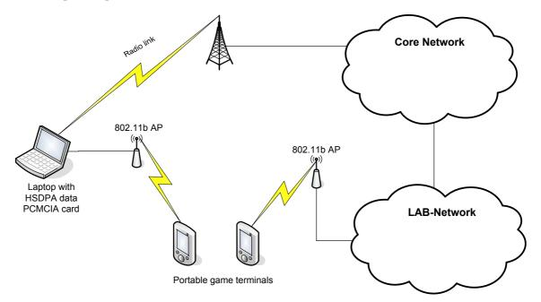
Figure 39. Laboratory setup for establishing a PSP multiplayer session over HSDPA
