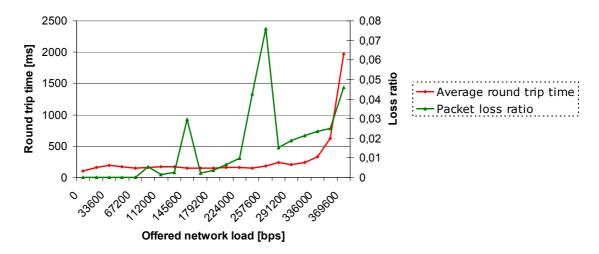
Figure 31. Large packet traffic's influence in an UMTS network
