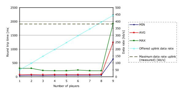
Figure 33. Multiple gamers influence on the latency over a single HSDPA connection
