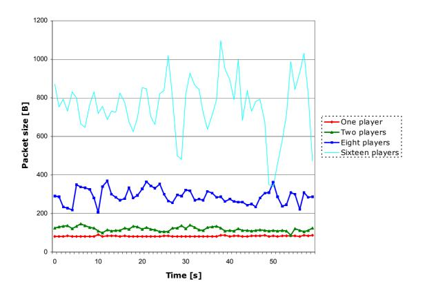
Figure 23. Quake 4 downlink packet size with varying number of players
