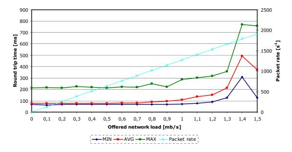
Figure 35. Small packet traffic's influence in an HSDPA network
