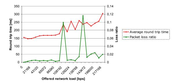
Figure 29. Small packet traffic's influence in an EDGE network
