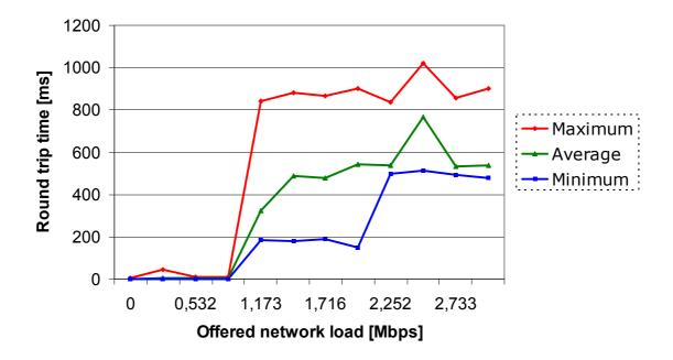
Figure 38. Small packet traffic's influence on an IEEE 802.11b access point
