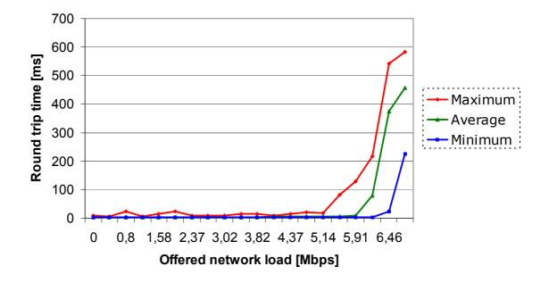
Figure 37. Large packet traffic's influence on an IEEE 802.11b access point
