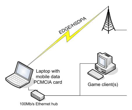
Figure 28. EDGE/HSDPA specific test setup
