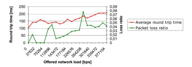
Figure 32. Small packet traffic's influence in an UMTS network
