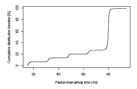
Figure 22. Quake 4 cumulative downlink packet inter-arrival time distribution
