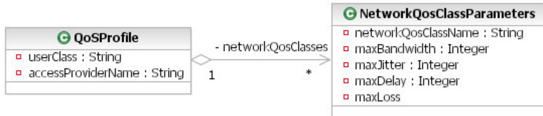
Figure 37: QoSProfile data structure
