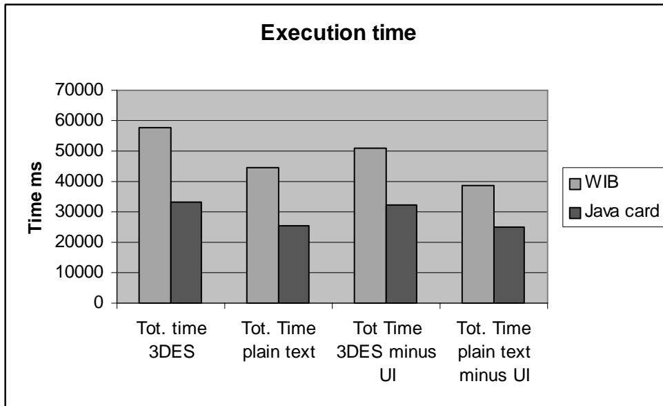
Figure 4-1 Comparison of the total execution time between the WIB and Java Card cases.
