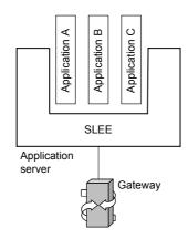
Figure 3.4: Service Logic Execution Environment, SLEE
