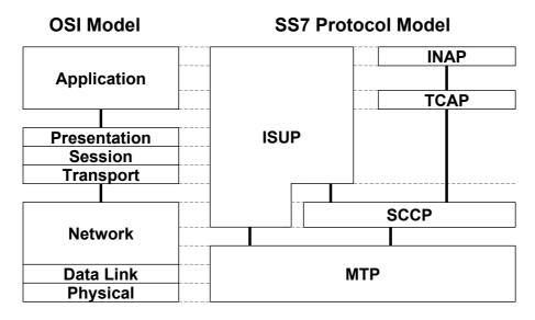
Figure 2.3: The SS7 protocol stack
