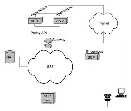
Figure 5.1: The Parlay gateway and interacting components
