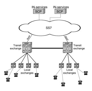
Figure 2.6: The Intelligent Network concept
