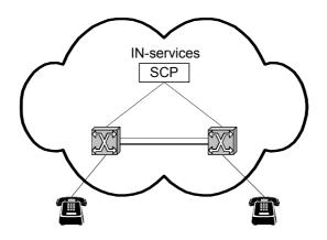
Figure 3.1: The centralised service architecture
