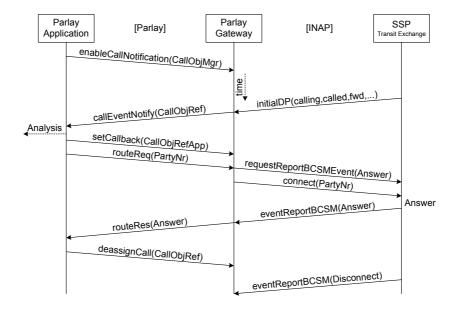
Figure 5.3: Web configured call forwarding sequence diagram
